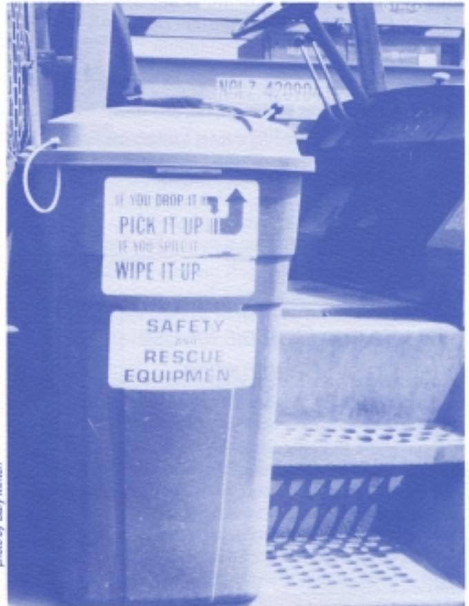
An innovative source control: this forklift carries a garbage can containing absorbent materials that could soak up spills.
