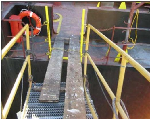
*Laying down wooden planks to span the open gap between the gangway and the deck does not ensure safe access.*
