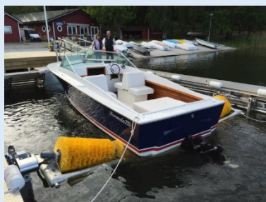
Figure 2: Motorboat being cleaned by a drive-in boat wash system.
