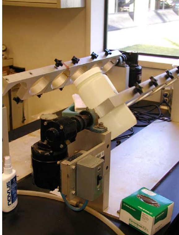
Figure 3-2. Rotary agitation device used for sample extraction in the TCLP and SPLP
