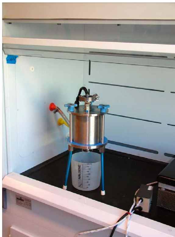
Figure 3-4. Filtration unit used for liquid/solid separation in the TCLP and SPLP when the sample is being tested for nonvolatile constituents
