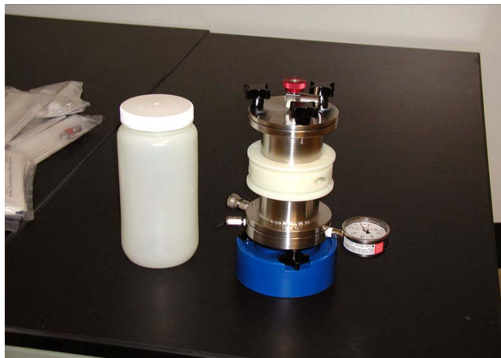
Figure 3-3. Zero-Headspace Extractor (ZHE) used for liquid/solid separation, extraction, and filtration in the TCLP and the SPLP when the sample is being tested for volatile analytes
