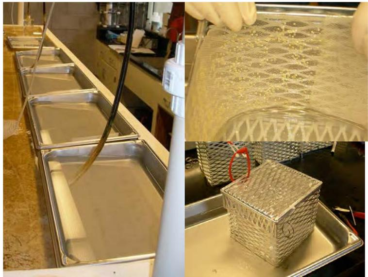
Figure 1. Egg fertilization and cage construction in the laboratory. Clockwise from left: replicate Nitex mesh sheets with monolayers of eggs incubating in milk; insertion of Nitex sheet with fertilized eggs into cage; fully assembled cage, or CESU. Photo courtesy of John Incardona, NOAA Fisheries.
