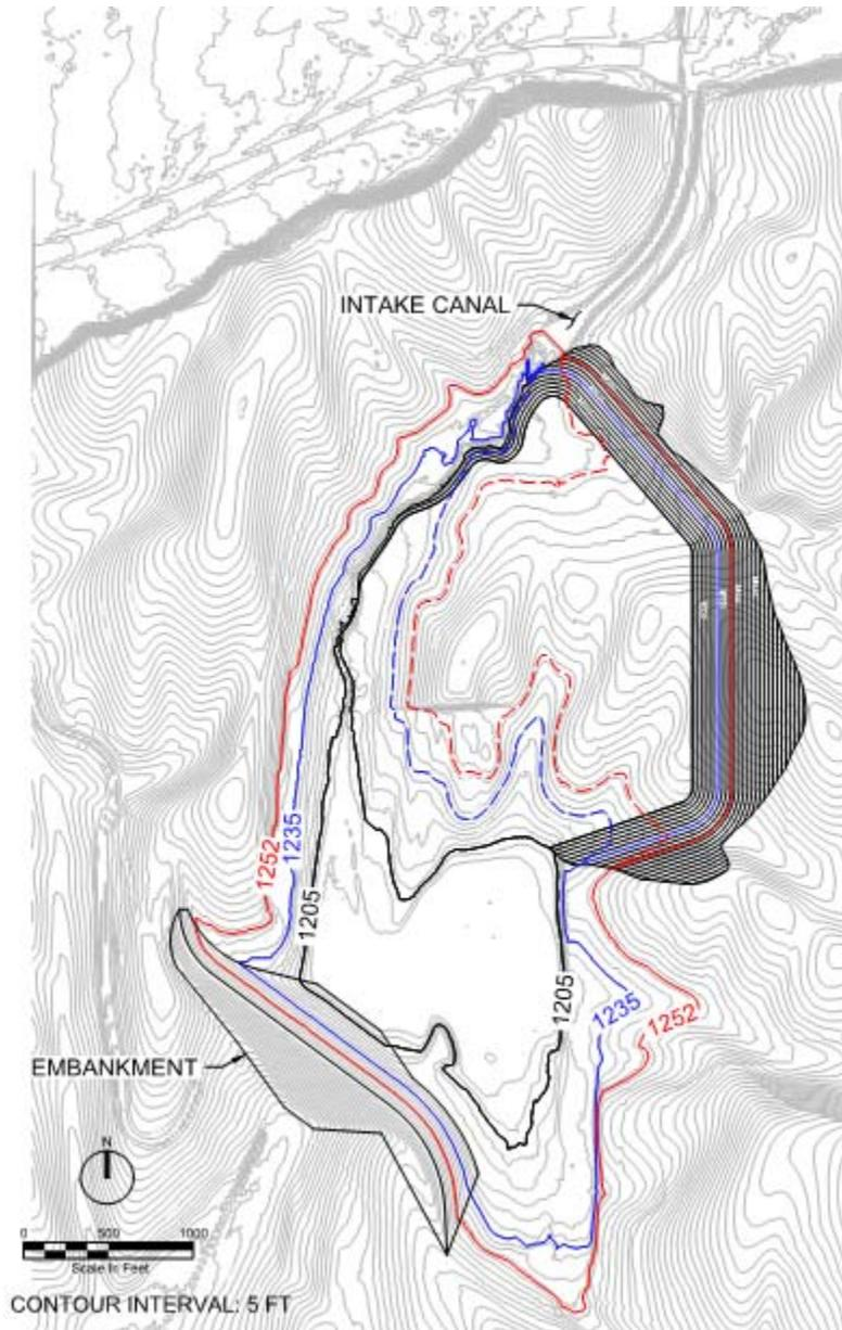
**Figure 1. Topographical Map of Bennington Lake with the Excavation for the Enlargement**
