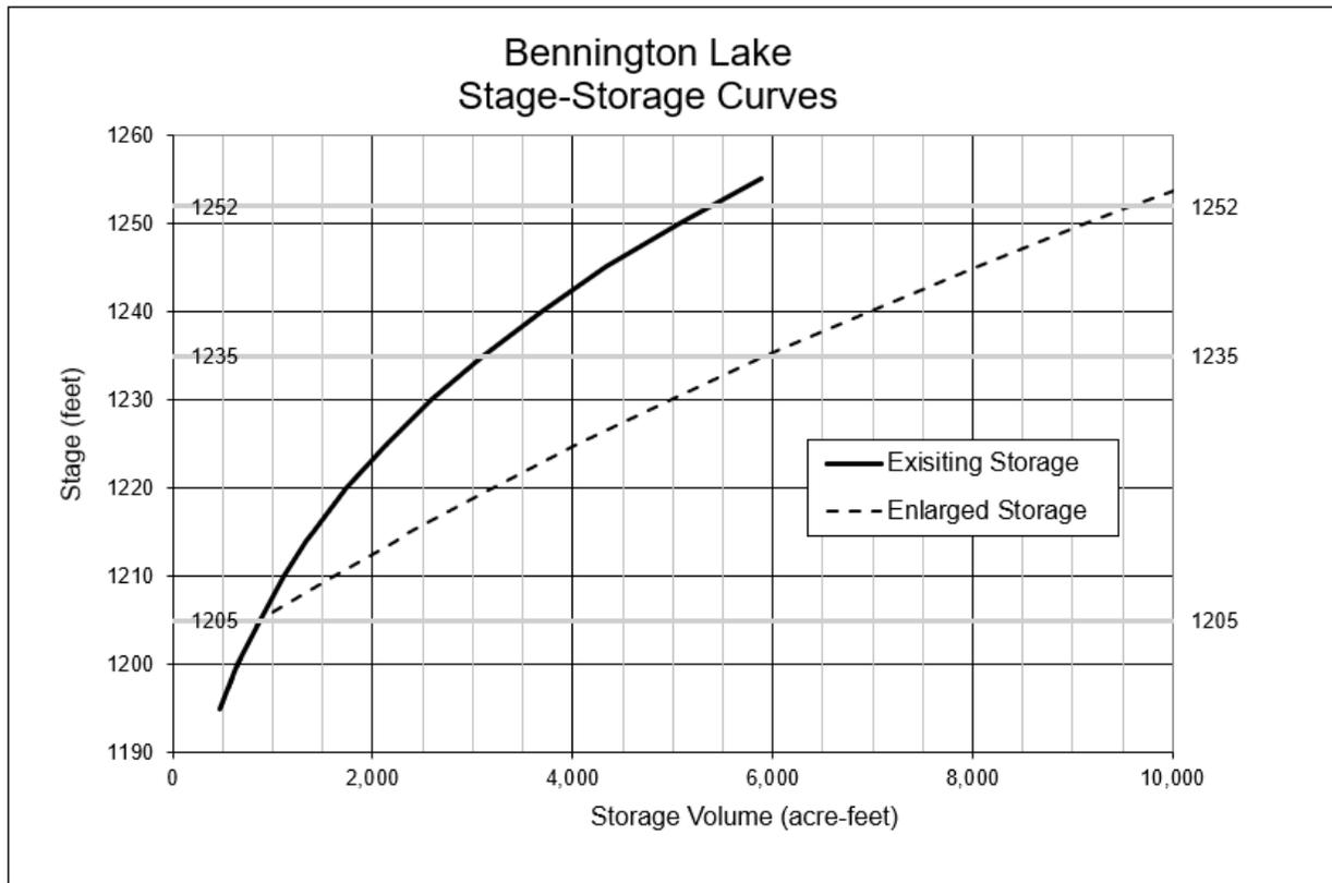
**Figure 2. Stage versus Storage for Existing and an Enlarged Bennington Lake**
