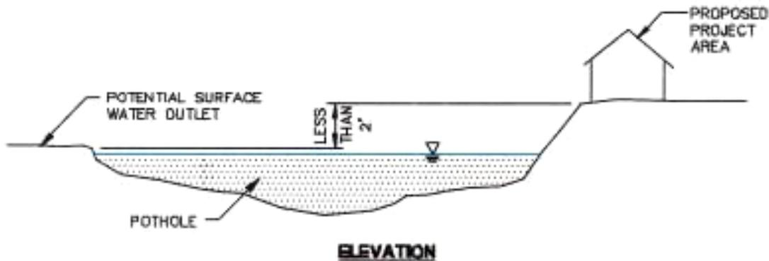
NOTE: AS SHOWN ABOVE, AREAS LOCATED WITHIN 2' OF VERTICAL HEIGHT OF A POTENTIAL SURFACE WATER SPILLWAY FROM THE POTHOLE ARE WITHIN THE POTENTIAL FLOOD HAZARD AREA
