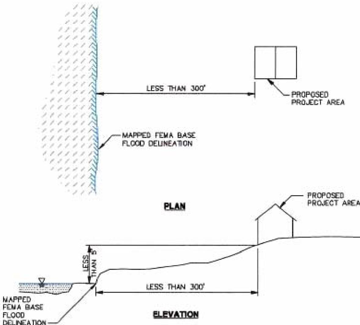
NOTE: AS SHOWN ABOVE, AREAS LESS THAN 300' HORIZONTAL DISTANCE FROM THE MAPPED FEMA BASE FLOOD DELINEATION, AND AREAS LESS THAN 5' VERTICAL HEIGHT ABOVE THE ESTABLISHED BASE FLOOD ELEVATION, ARE WITHIN THE POTENTIAL FLOOD HAZARD AREA
