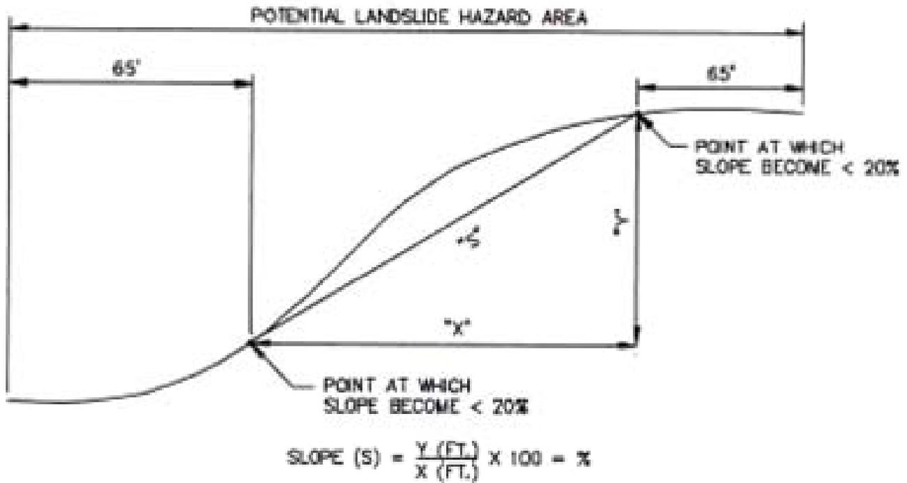
**POTENTIAL LANDSLIDE HAZARD AREA - SLOPES
