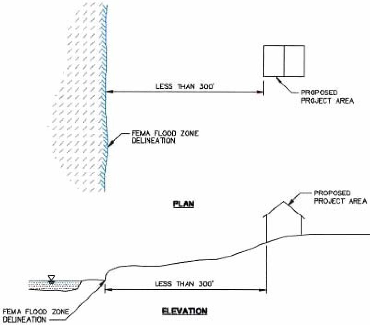
**NOTE:** AS SHOWN ABOVE, AREAS LESS THAN 300' HORIZONTAL DISTANCE FROM THE MAPPED DELINEATION OF THE FEMA FLOOD ZONE ARE WITHIN THE POTENTIAL FLOOD HAZARD AREA.
