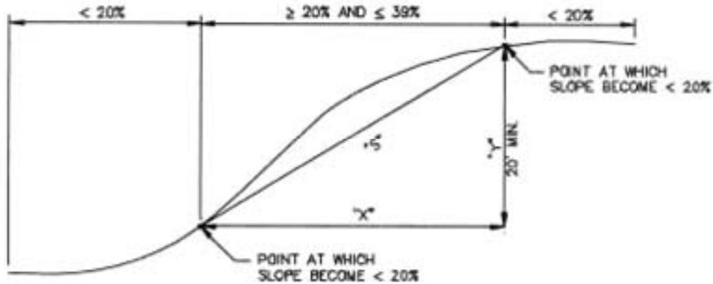
$$\text{SLOPE (S)} = \frac{Y \text{ (FT.)}}{X \text{ (FT.)}} \times 100 = \%$$
