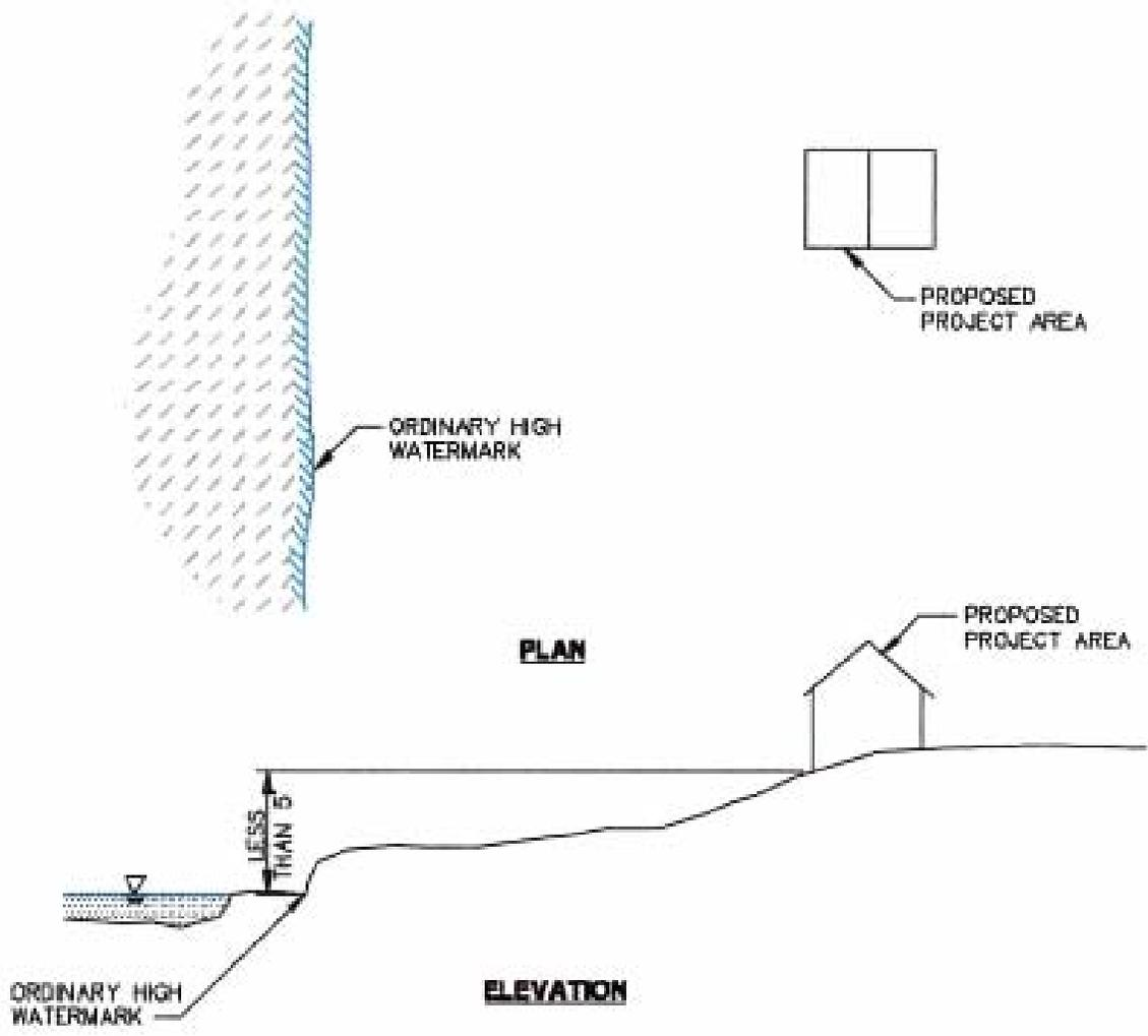
**NOTE:** AS SHOWN ABOVE, AREAS LESS THAN 5' VERTICAL HEIGHT ABOVE THE ORDINARY HIGH WATER MARK OF AN IDENTIFIED NATURAL WATER ARE WITHIN THE POTENTIAL FLOOD HAZARD AREA.
