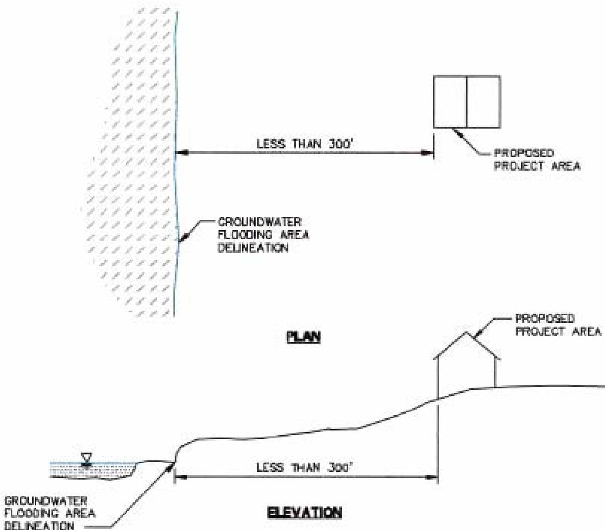
NOTE: AS SHOWN ABOVE, AREAS LESS THAN 300' HORIZONTAL DISTANCE FROM THE MAPPED DELINEATION OF A GROUNDWATER FLOODING AREA ARE WITHIN THE POTENTIAL FLOOD HAZARD AREA
