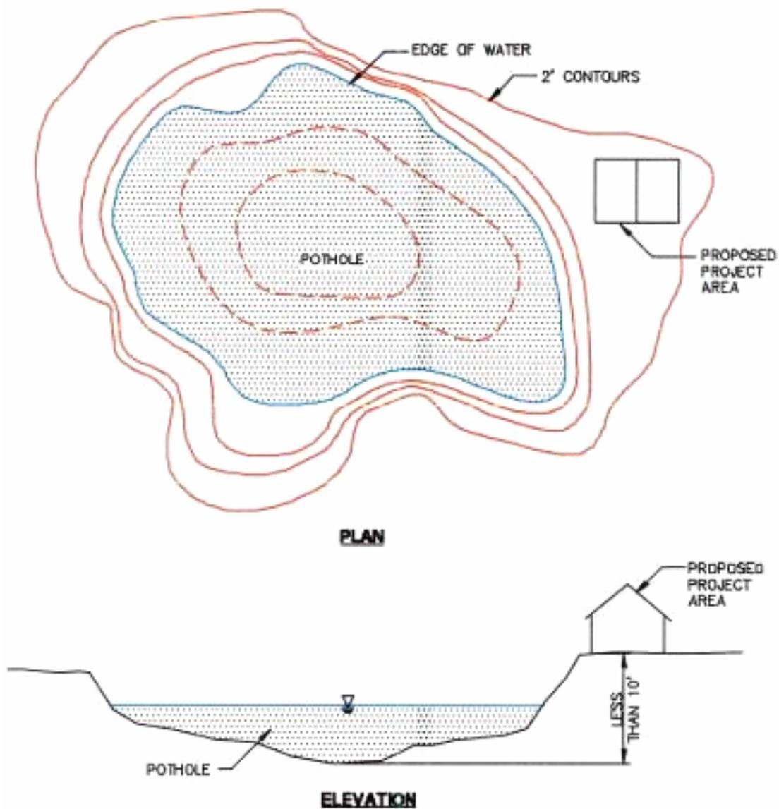
**NOTE:** AS SHOWN ABOVE, AREAS LOCATED WITHIN 10' OF VERTICAL HEIGHT FROM THE BOTTOM ELEVATION OF AN IDENTIFIED POTHOLE ARE WITHIN THE POTENTIAL FLOOD HAZARD AREA.
