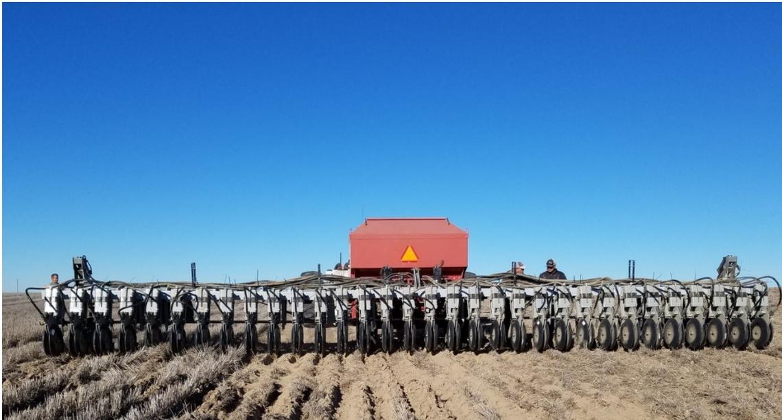
**Figure 8: Deep furrow conservation drill prototype**
